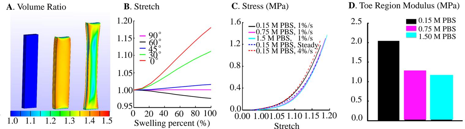
**Fig. 3.** (A) Tissue ( $\pm 60^\circ$  fiber) before testing (left), during swelling (0.15M PBS; center) and under tension (right). (B) Fiber stretch during swelling with respect to fiber angle orientation. (C) Tensile stress-stretch behavior with respect to osmolality and loading rate. (D) Toe-region tensile modulus of tissue ( $\pm 60^\circ$  fiber) after swelling in different osmolality PBS.
