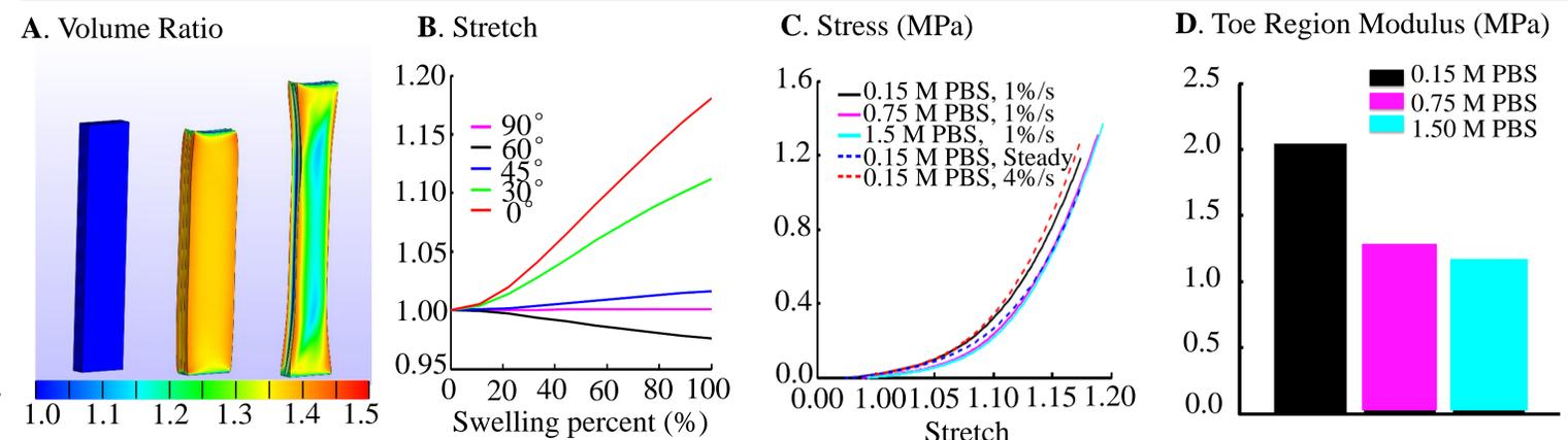
**Fig. 3.** (A) Tissue ( $\pm 60^\circ$  fiber) before testing (left), during swelling (0.15M PBS; center) and under tension (right). (B) Fiber stretch during swelling with respect to fiber angle orientation. (C) Tensile stress-stretch behavior with respect to osmolality and loading rate. (D) Toe-region tensile modulus of tissue ( $\pm 60^\circ$  fiber) after swelling in different osmolality PBS.
